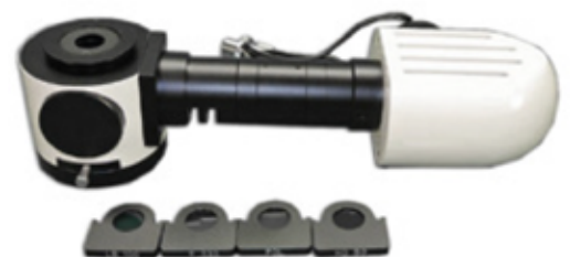
MA927 VERTICAL KOEHLER ILLUMINATOR WITH HALOGEN LAMP 6V, 30W AND FILTERS
